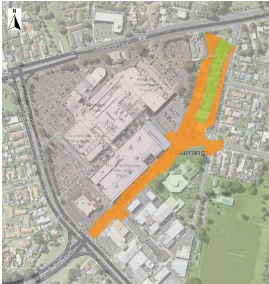
Figure 29: Indicative work zones – Reeves Rd and RRF
